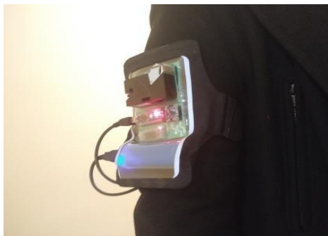
Figure 2. Wearable device based on CCS811 sensor worn on the user's arm for personal air quality monitoring. (Source: Géczy et al., 2022)
