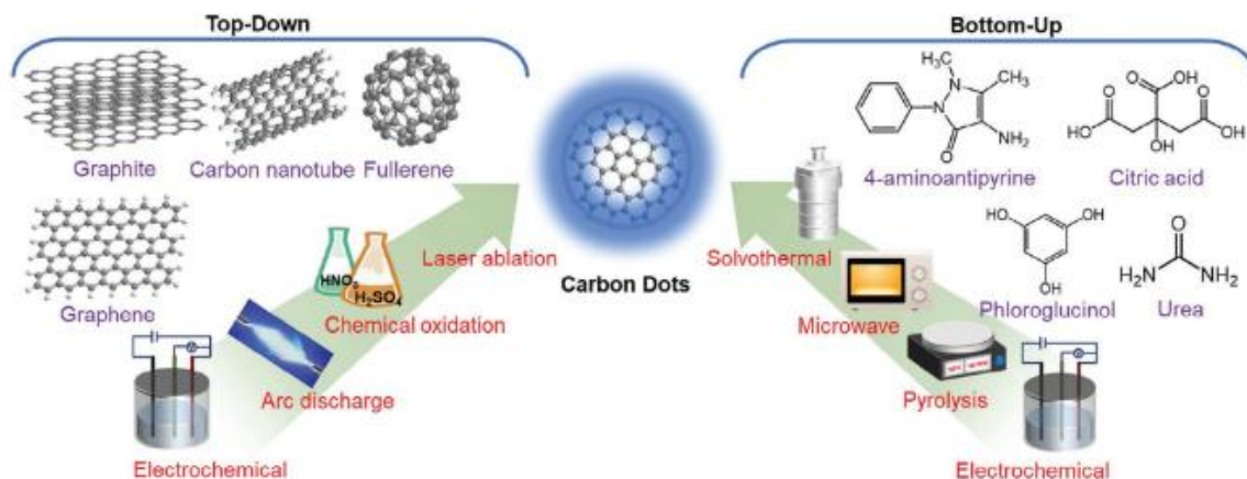
Figure 1. Synthesis methods for Carbon Nanodots (CNDs) (Ren et al., 2024)
